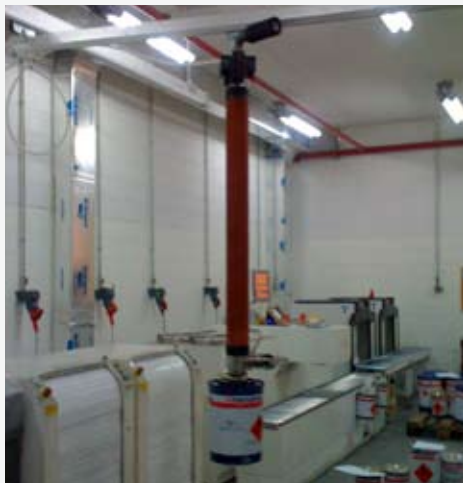
4. ATEX zon 1 installation, ejektordriven VM120, standard sugfot art nr 630215.
